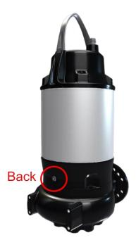
Install the motor on the volute so that the front drain plug is in line with the discharge of the volute. Now make sure that the lifting handle is oriented correctly. The handle has a longer sloping side and a shorter sloping side. The longer side should point towards the discharge of the volute (the front). Installing the handle backwards may lead to issues when using the pump on an autocoupling system.
