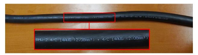
Cable size is printed on the cable above as "4/C 14AWG + 4/C 14AWG." This means this cable has Qty.4 14AWG Power leads and Qty.4 14AWG Control leads. RHW power cables have Qty.4 Power leads of different sizes and Qty.4 14 AWG Control leads. E.G., 4x10+4x14, 4x4+4x14. If there are 8 leads in the cable, it is RHW cable. (Note: some arrangements may use a Qty. 12 16AWG SOOW Control cable in addition to the power cable and smaller pumps may only use a Qty. 4 14AWG SOOW cable)
