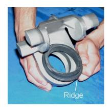
Press the seal into its seat starting on one side and work the rest of the seal into the same position. When finished, it should look as below.
