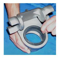
When properly installed, the profile seal will stay in place when pulled straight outwards.
