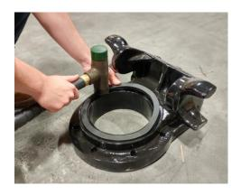
If the seal goes in easily, it is most likely backwards. When installed properly, the seal forms a "dovetail" with the claw.
