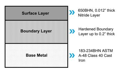
surface layer of the metal which increase the hardness, as well as diffuse into the part to create a boundary layer between the base metal and the nitride layer. This results in a thin, hardened surface without the brittleness of through-hardened materials.
